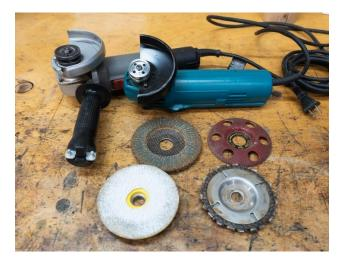
I have found the Mini Arbortec to be many times safer than the Lancelot or 4" Arbortec. The reason is its simply smaller and cuts so easily that catches are almost non existent. It does take a range of cutters. This tool is very easy to control.
