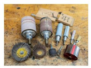
Scotch Brite radial bristle discs are incredibly useful for cleaning up finer details. Also very good for softening sharp edges and cleaning up little fibers left from Carbide burrs.
