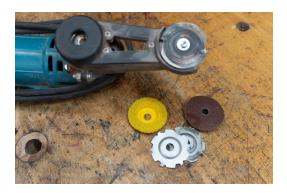
The Foredom and other flex shaft machines take a wide range of cutters and sanding drums. This is a very flexible tools because you can also get a reciprocating handpiece that allows carving with gouges and other shaped edge tools. I like the rotary burrs because they have a very short learning curve and are pretty safe to use.
