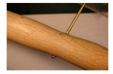
Now I insert the brass rod. I put medium CA glue or epoxy into the hole and a little on the brass rod. Then I drive it through the hole.
