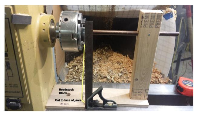
Make an upright and mount it to a piece of wood. Drill a hole in the upright at center line of your lathe. With the foot against the headstock block insert and glue a dowel until it is aligned with the face of the chucks jaws.
